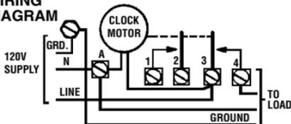
TYPICAL WIRING: SINGLE POLE NORMALLY OPEN
