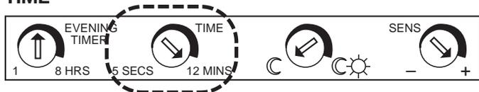
Sets the time that lights will remain on after the detection zone is vacated. Adjustable from approximately 5 seconds to 12 minutes. The Factory Setting is 12 minutes.
