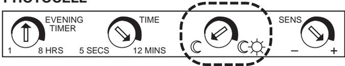
For night-only operation, turn the knob completely counterclockwise to (to the MOON symbol). For 24-hour operation turn the knob all the way clockwise to the MOON/SUN symbol. Adjust counterclockwise to have the sensor come on later at dusk, clockwise to have it come on earlier. The Factory Setting is Night-only (MOON). If you set Evening Timer while set to 24 hour operation, Evening Timer will begin immediately after flipping switch.
