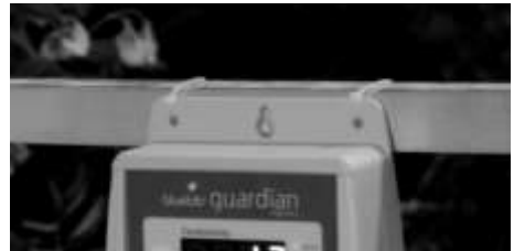
Cable ties fixed through small mounting holes around a support or bar
