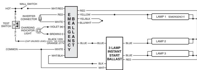
FIG 105 THREE (3) LAMP RAPID START BALLAST
