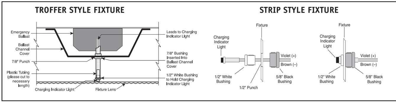
NOTE: After installing the charging indicator light and test switch, mark each with the appropriate label.
