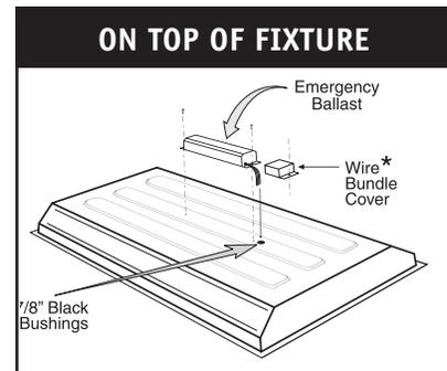
\* For installation on top of the fixture, wire bundle covers (RMC-60) may be required by state or local codes. These covers are available from the manufacturer as an accessory kit and must be ordered separately. Call your local distributor or the factory for complete information.
