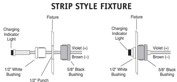
**NOTE:** After installing the charging indicator light and test switch, mark each with the appropriate label.
