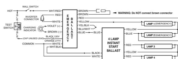
**WIRING DIAGRAMS for Emergency-Only fixtures**
