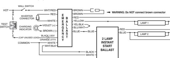
FIG 140 TWO (2) LAMP RAPID START BALLAST
