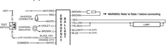
FIG 110 TWO (2) 17-40 W LAMPS WITHOUT AC BALLAST
