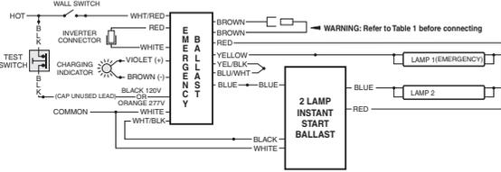
FIG 133 TWO (2) LAMP RAPID START BALLAST
