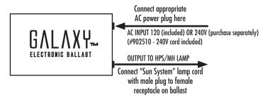
These ballasts offer our exclusive Smart Volt™ feature — They are "smart" ballasts — They will operate on either 120 or 240 volt power (except Galaxy™ 1000 watt 240 volt only ballast, part #902510) by simply plugging in the appropriate power cord. There is no further modification necessary. It comes with a 120 volt power cord. If you wish to run this ballast on 240 volt, you must purchase the 240 volt power cord separately (part #903082 six foot or #903084 twenty foot).
