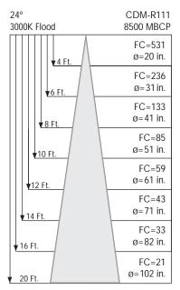
Beam spread at 50% Maximum Beam Candlepower—0° primary angle FC=Footcandles at mounting height ø=Beam diameter at mounting height
