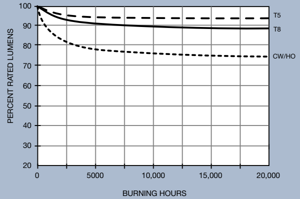
Fluorescent Lamp Lumen Maintenance
