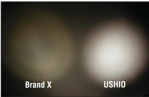
Brand X – Uneven beam pattern, low color temperature, green color and low output
