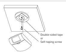
Sensor mounts under desk or binder bin with double-sided tape or self-taping screw
