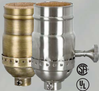
METAL SHELL 3-WAY BRASS ELECTROLIER HAND POLISHED & LACQUERED LO-MED-HI-OFF FOR USE WITH 3-WAY LAMP SOLID BRASS REMOVABLE TURN-KNOB BUSHING TAPPED 1/8 IPS RATED 250W – 250V D3855 ANTIQUE BRASS D3857 SATIN NICKEL
