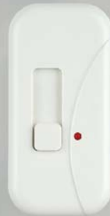
IVORY FEED THRU SLIDE DIMMER SPT-2 WIRE - INCANDESCENT ONLY W/ LED NIGHT LIGHT 120V - 300W D5892
