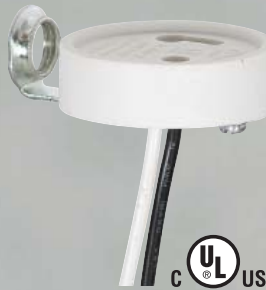
GU24 SOCKET WITH SIDE HICKEY 18" AWM 105° LEADS RATED 600V – 660W D3512
