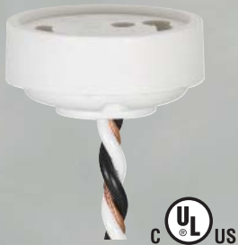
GU24 SOCKET 1/8F • WITH GROUND WIRE 18" AWM 105° LEADS RATED 600V – 660W D3516
