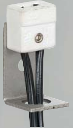
CERAMIC WEDGE BASE SOCKET STAINLESS STEEL BRACKET SLIPS 1/8 IPS 3/16" SIDE HOLE D2606 9" 200°C LEADS D2608 36" 105° SPT-1 LEADS
