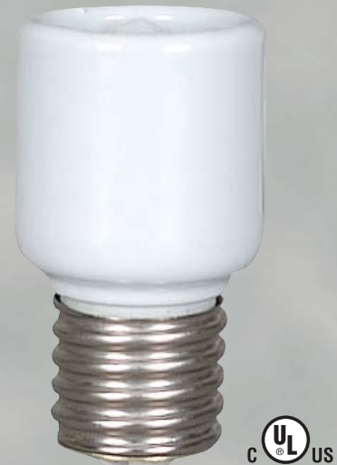
MOGAL TO MOGAL 4 KV PULSE RATED GLAZED PORCELAIN SOCKET EXTENSION FOR USE WITH HIGH INTENSITY DISCHARGE LAMPS • COPPER ALLOY, NICKEL-PLATED SCREW SHELL RATED 1500W – 600V D348
