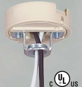
GU24 SOCKET MOUNTING BASE WITH 1/8F "U" HICKEY #8/32 SCREW HOLES 18" AWM 105° LEADS RATED 600V – 660W D3519
