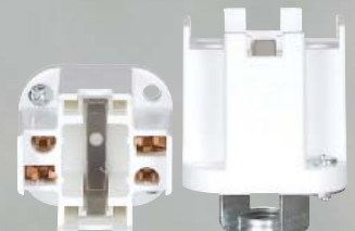
SOCKET WITH HICKEY FOR G24Q-1 & GX24Q-1 LAMP BASES 13 WATT 4-PIN CFL 1/8 IPS HICKEY D2740
