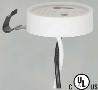
GU24 SOCKET WITH SIDE CLIP 18" AWM 105° LEADS RATED 600V – 660W D3511
