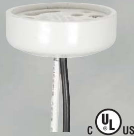
GU24 SOCKET 1/8F • LOCKING FEATURE 18" AWM 105° LEADS RATED 600V – 660W D3513
