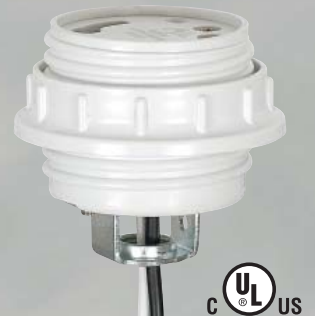
GU24 SOCKET WITH LOCKING FEATURE 18" AWM 105° LEADS RATED 600V – 660W D3514
