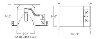
Cut out: 6-3/4" Height: 7-1/2" Housing Length: 13-1/4" Housing Width: 9-1/2"
