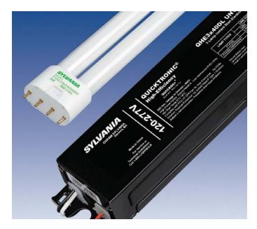
SYLVANIA DULUX L SUPERSAVER lamps are high-lumen, single-ended twin-tube lamps that provide lumen output similar to 4' linear fluorescent lamps, yet are half the length. With up to 2800 lumens and lamp efficacy up to 100 lumens per watt, these compact fluorescent lamps can be used in both direct and indirect lighting applications.
