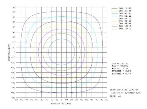
C Range: 0 - 360DEG C Interval: 22.5DEG Test Speed: HIGH Temperature:25.1DEG Operators:Jack Test Date:2012-02-21
