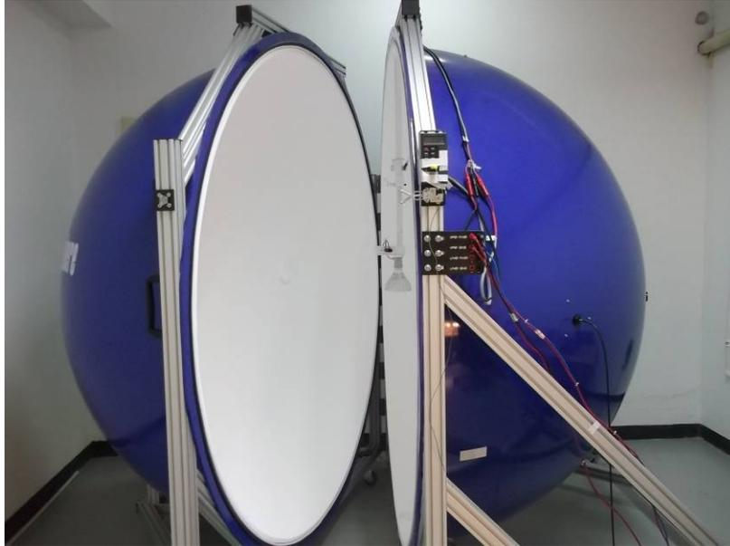
Figure 2: Testing in Integrating Sphere
