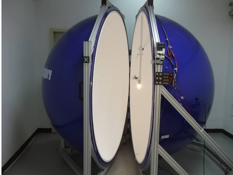
Figure 2: Testing in Integrating Sphere
