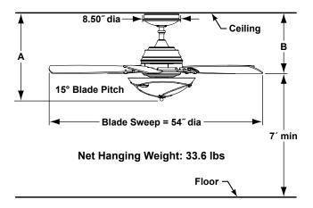
Fan must be attached to a securely anchored electrical junction box capable of withstanding a load of at least 50 lbs.
