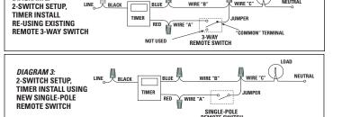
NOTE: For new construction or to replace a dimmer switch, a lighted switch, or a 3-way switch without screw terminals, a single-pole switch can be used at the remote location, as
