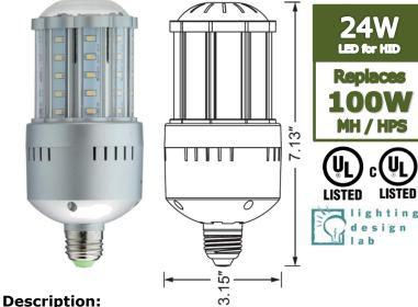
24W LED retrofit lamp to replace MH and HPS lamps up to 100w, E26 Medium base. Integrated insect/dust screen. UL damp rated approved for fully enclosed fixtures.
