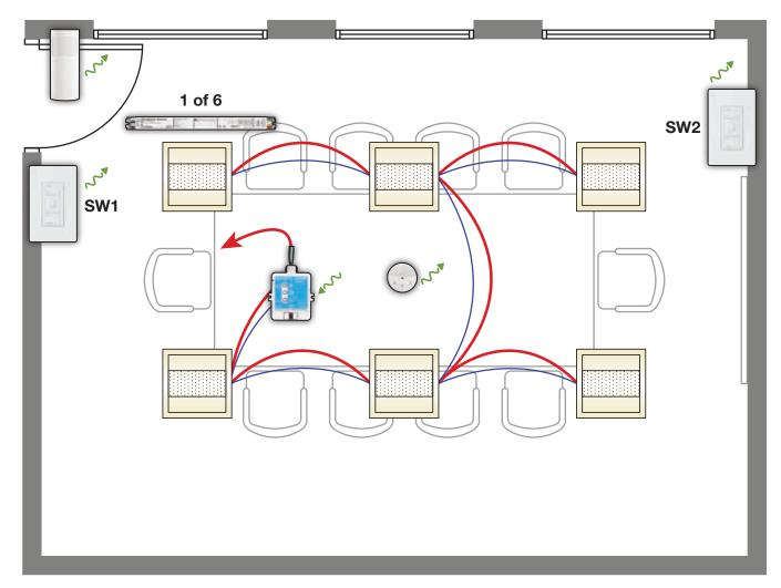
Line voltage wiring Low voltage wiring ✓ Clear Connect<sub>®</sub> **RF Communication**
