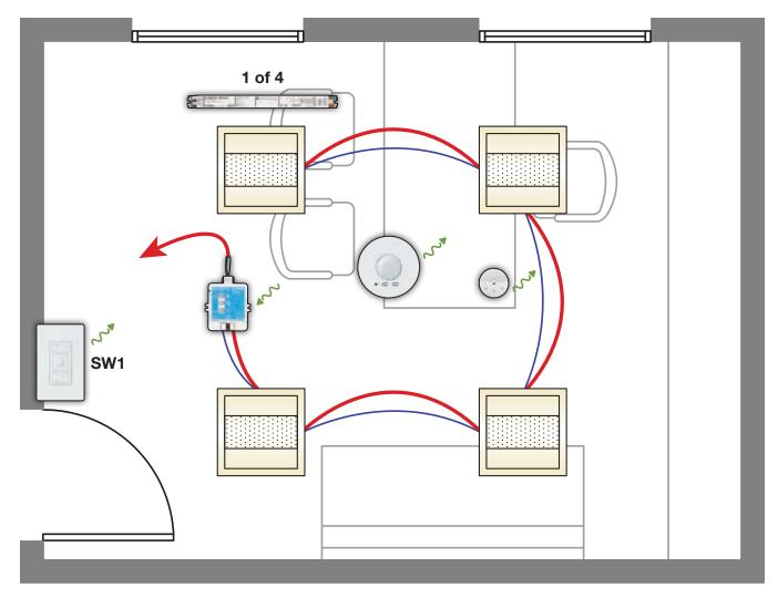
Line voltage wiringLow voltage wiring
