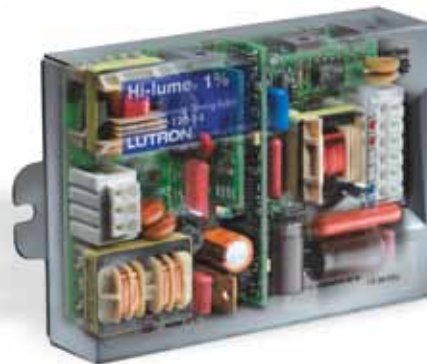
Components in a Hi-lume® 1% dimming ballast for compact fluorescent lamps
