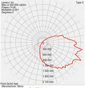
Luminaire catalog: Large Cuttoff Wallpack Luminaire: Wallpack With Prismatic Glass Lens Lamp catalog: 64 XBDs. LUMINAIRE OUTPUT = 5893 LMS Lamp: Two LED arrays with 32 LEDs each
