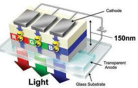
OLED is a solid-state semiconductor device composed of ultra-thin films of organic molecules that create light.
