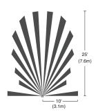
The WN-100 has a coverage range of 180° and a maximum coverage area of 300 ft². To maintain its coverage capacity and optimally detect motion, the WN-100 must have a clear and unobstructed view of occupants.
