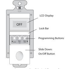
To access setup buttons gently pull the Lock Bar away from the switch face and slide the ON/OFF button down. (RT-100)
